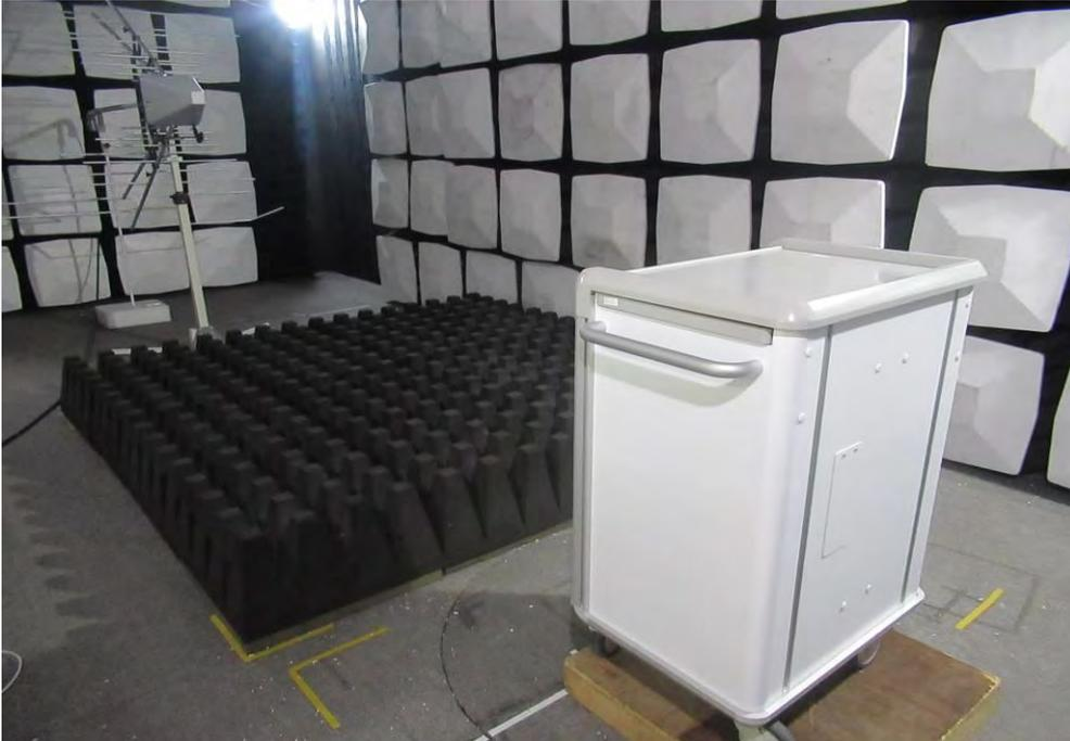
Electrostatic Discharge Measurement Test Setup Photos (EN 61000-4-2)
